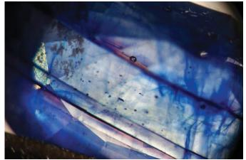
Figure 11. When viewed with transmitted light field illumination, rich blue colour concentrations are found in the fissures. Photo by Wimon Manorotkul.
