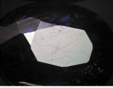
Figure 18. Table facet of one cobalt-doped glass-filled sapphire before (top) and after (below) heating with a jeweler's torch. Photos by Thanong Leelawatanasuk.
